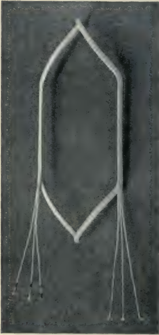
FIG. 308.—Three-turn Wire-wound Armature Coil.
